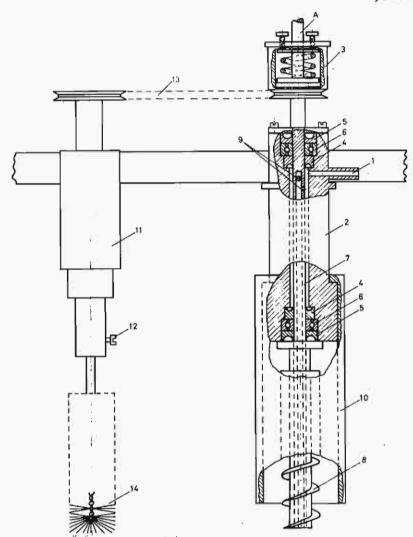
In order to clean Drosophila culture tubes in relatively short time, we have developed a cleaning device which is in operation in our laboratory since a year and proved to be very helpful.
